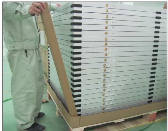
4 carton protections are inserted at each corner to strengthen and protect the pallet
