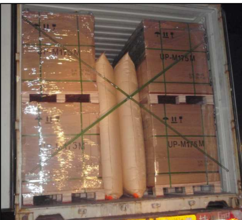
Once the container is full, air bags are inserted to maintain pallets in position
