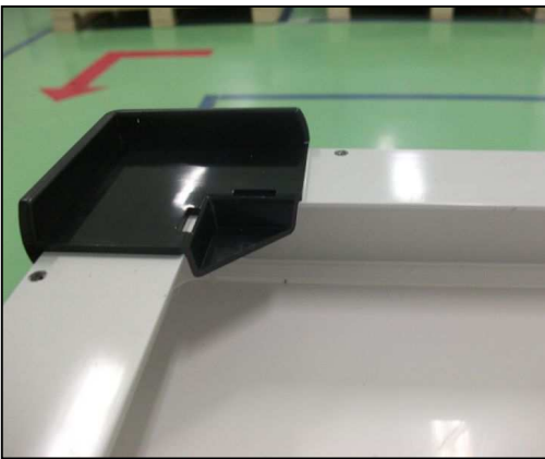
6 ABS pieces are fixed on each frame to avoid any contact between 2 modules
