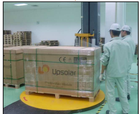
Each finished pallet is wrapped in plastic film to ensure the pallet integrity
